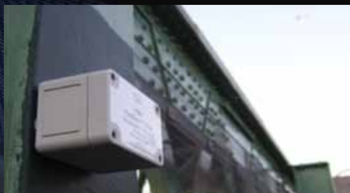
Senceive: Bridge monitoring (Network Rail)
